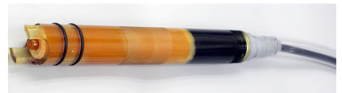
Side view of WPITC CPVC submersible option sealing assembly
