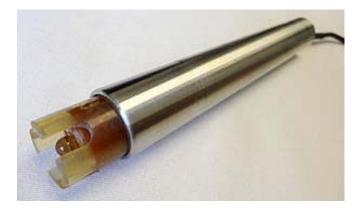
5731 Aggressive Dissolved Gas & Solvent Resistant pH sensor Close-up view of tip with 4 each "GR" thick protective tines Double sealing O-rings for integrity & safety of installation Ideal for organic manufacturing processes employing volatile solvents& pressurized vessels requiring safe HOT-TAP use Standard Viton®-75 O-rings with CV75, Simriz® 485 & Kalrez® 4079 optional as required
