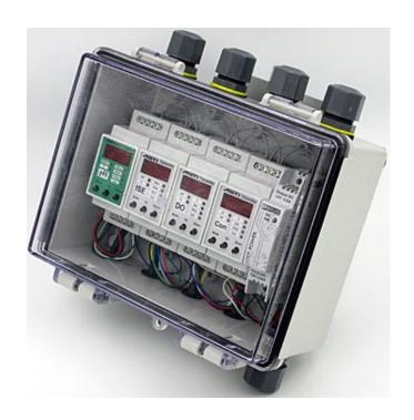
Quad channel transmitter assembly in NEMA 4X rated 5MF enclosure. For measurement of pH with smart digital sensors and for measurement ion selective, dissolved oxygen and conductivity parameters with analog sensors. Any mix of smart digital and analog sensors can be used with the 3TX-HiQ & 3TX transmitter platforms, respectively.
