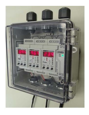
Triple Channel Nitrate, pH & Conductivity Transmitter 3TX-3MF-ISE-NO3-D-pH-D-CON-1.0/50-D-PS
