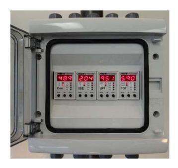
Triple Channel Total Ammonia, pH & Conductivity Transmitter 3TX-4M-ISE-NH4-A-pH-A-TOT-CON-1.0/50-A
