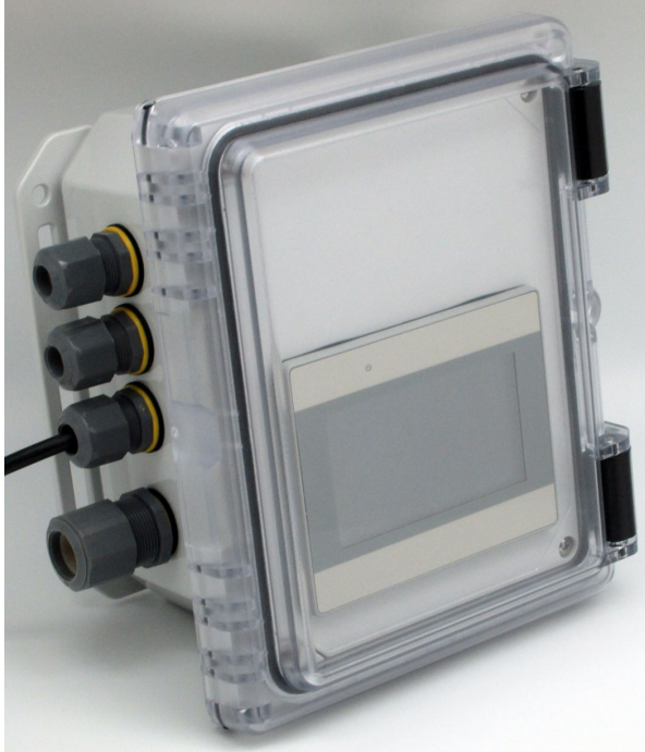
Dual (2) channel RTU touchscreen controller shown above on right with 2 each waterproof HiQ4FP panel mount ports on right input side for the HiQDT smart digital RS485 MODBUS RTU pH sensors. On left above four (4) cable glands on left output side for power, output & ethernet cable. Controller is NEMA 4X when the door is latched. Hot swappable smart plug & play sensors come with NEMA 6P rated HiQ4M snap connectors.
