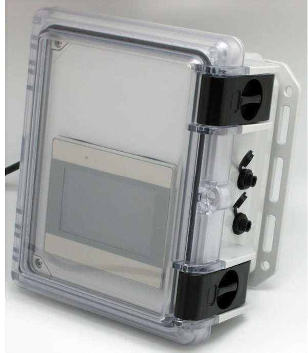
Dual (2) channel RTU touchscreen controller shown above on right with 2 each waterproof HiQ4FP panel mount ports on right input side for the HiQDT smart digital RS485 MODBUS RTU pH sensors. On left above four (4) cable glands on left output side for power, output & ethernet cable. Controller is NEMA 4X when the door is latched. Hot swappable smart plug & play sensors come with NEMA 6P rated HiQ4M snap connectors.
