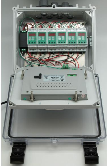
Photo above for fully populated six channel touchscreen controller assy. Large seven (7) inch touchscreen for configuration of channels, output scaling, calibration & display for all sensors. The isolated analog output provided from each 3TX-RTU-D transmitter. The digital MODBUS TCP output is provided from the ethernet port on the HMI.
