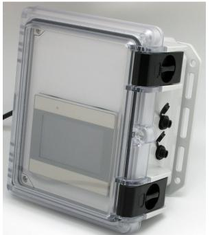
*Dual (2) channel RTU touchscreen controller shown above on right with 2 each waterproof HiQ4FP panel mount ports on right input side for the HiQDT smart digital RS485 MODBUS RTU pH sensors. On left above four (4) cable glands on left output side for power, output & ethernet cable. Controller is NEMA 4X when the door is latched. Hot swappable smart plug & play sensors come with NEMA 6P rated HiQ4M snap connectors.*
