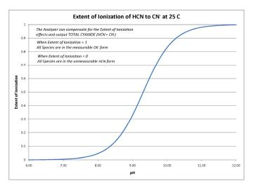
The 3TX-TOT module uses built-in algorithms to compute the extent of ionization for the system of interest ( $NH_3$ , HF, HCN) at the current pH and temperature. The Total ISE is found by simply taking the Free ISE and diving it by this computed extent of ionization. The resulting Total ISE shows what would be the ion activity detected if all of the species were in the measurable form.
