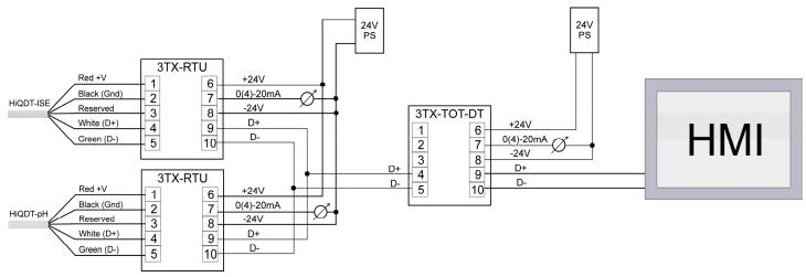
Node Address for **3TX-RTU-D** Transmitters with Six Channel Touchscreen Controllers (Channels 4, 5 & 6 are not used in this configuration but can be added at a later time)
