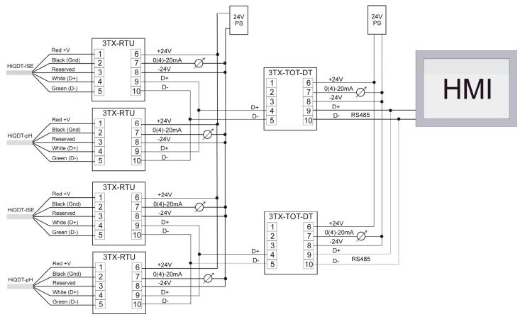
*NOTE:* The two total ISE installations measured in the configuration detailed in the wiring schematic above can be either redundant (two sets of ISE & pH sensors in the same tank or line) or from two separate installation points or locations as preferred.
