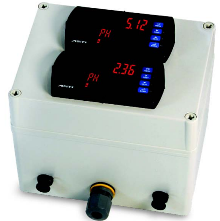
Dual Channel HiQDT-NEMA4X-LEDTX Controller in Master Configuration shown without sensors. Waterproof caps should be affixed when sensors are not connected. Cable glands are factory installed on top of enclosure for sealing analog output and contact relays connections (not visible from bottom view angle in photos shown above).
