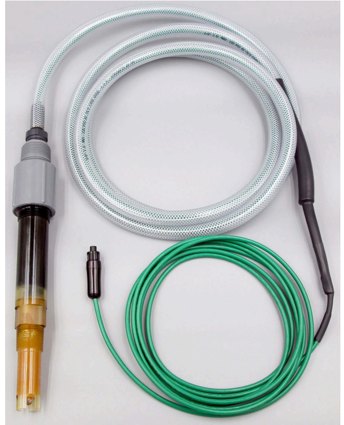
PNHF 6431-HiQ-WPH/10 Fully Submersible Acid/Fluoride High HF Resistant Smart Digital pH Sensor with WPH waterproofing seal, 6 meters (20 feet) of integral cable & 3 meters (10 feet) of braid-reinforced vinyl tubing; Typical applications include acid fluoride etching control & monitoring or industrial wastewater treatment (WWT) plants
