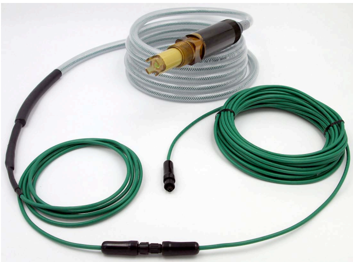
Smart Digital ZEUS pH Sensor (Item # 1205) with 12 meters (40 feet) female snap to male snap extension cable shown interfaced; Max rating of 150 °C @ 200 psig, Fully Submersible to 12 feet, Typically uses include processes with dissolved ammonia, chlorine, sulfides & abrasive slurries
