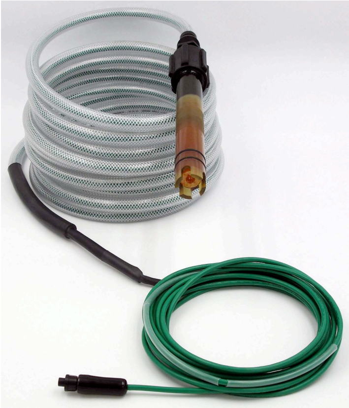
PNXGRE 5631/5331-HiQ-12m-WPB/20 Submersible Sulfide & Slurry/Viscous Resistant Smart Digital pH Sensor with Extreme Dehydration Resistant Junction for Intermittent Wet and Dry Use, 12 meters (40 feet) of integral cable & WPB with 6 meters (20 feet) of reinforced vinyl tubing for installs down in a sewer through a manhole
