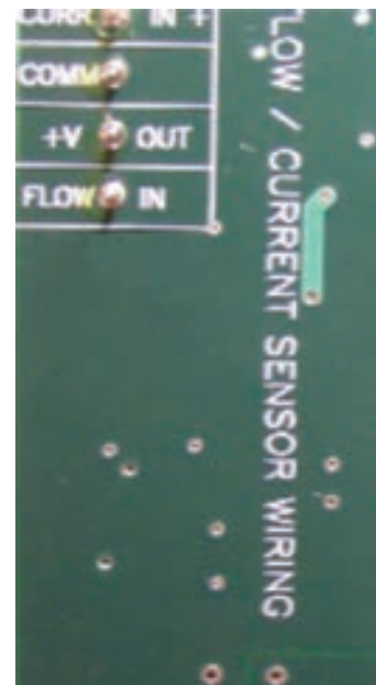
Figure 3-11 Flow/Current Input signal board and Sensor cable leads
