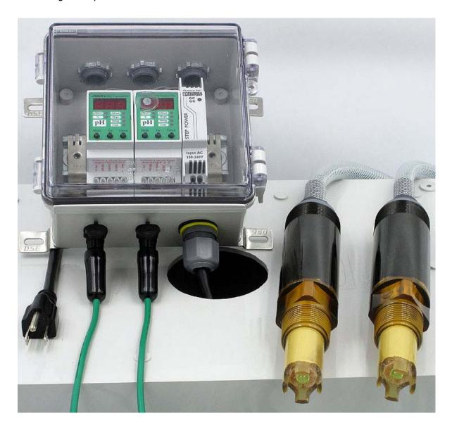
ZEUS™ pH Sensors in Smart Digital Configuration with NEMA 6P rated HiQ4M cable connector (Item # 1205)
