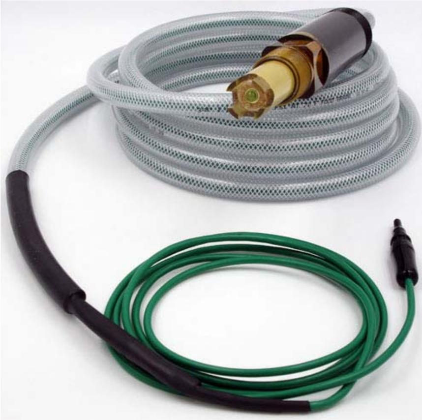
*ZEUS™ pH Sensor in Smart Digital Configuration with 20 feet cable assembly complete, submersible to 12 feet. Shown with protective cap installed on NEMA 6P rated quick disconnect snap connector termination as shipped from factory.*
