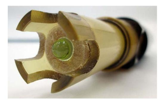
Close-up of ZEUS $^{\text{\tiny M}}$  pH sensor measuring tip. Solid-state conductive polymer reference system (brown) is sealed to thick-wall break-resistant low-profile parabolic pH sensing element (green) protected by ultra-rugged 4 each protective tines for guard
