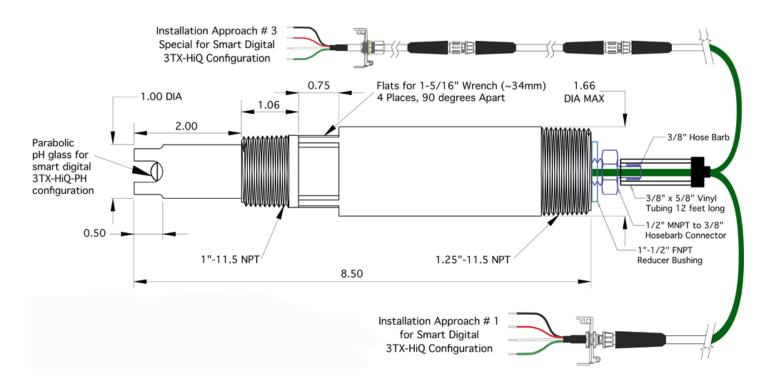
Selected Pictures for Visualization of ZEUS™ pH Sensor in the Smart Digital Configuration
