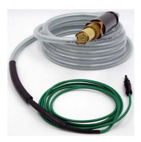
ZEUS $^{\text{\tiny M}}$  pH Sensor in Smart Digital Configuration with 20 feet cable assembly complete, submersible to 12 feet. Shown with protective cap installed on NEMA 6P rated quick disconnect snap connector termination as shipped from factory.
