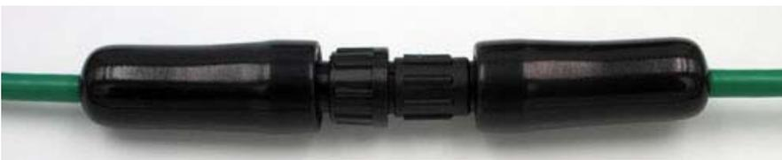
*Male Snap from ZEUS™ pH sensor in Smart Digital Configuration. Connected to Female Snap from Extension Cable NEMA 6P rated for use in aggressive field service*
