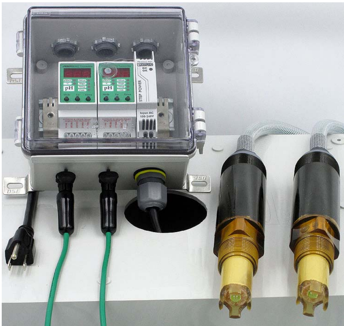
ZEUS™ pH Sensors in Smart Digital Configuration with NEMA 6P rated HiQ4M cable connector (Item # 1205) shown connected to dual channel 3TX-3MF-2H-2EA-HiQ-pH-PS intelligent digital pH transmitter (Item # 11305) via the receiving 2 each female panel mount HiQ4FP snap connector installed into 3MF NEMA 4X enclosure.
