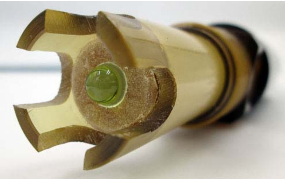
Close-up of ZEUS™ pH sensor measuring tip. Solid-state conductive polymer reference system (brown) is sealed to thick-wall break-resistant low-profile parabolic pH sensing element (green) protected by ultra-rugged 4 each protective tines for guard
