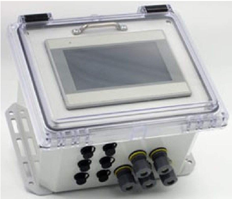
HiQDT-CTRL-6CH six channel controller with 7.0" touchscreen shown in lid closed position. For the triple channel configuration there would exist only 3 each of the HiQ4FP female panel mount connectors. All packages are NEMA 4X pre-installed with all necessary cable glands ready for field use.
