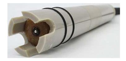
Model 5841 PEEK bodied sanitary ORP sensor shown with low-profile ball-style platinum ORP sensing element for use in high viscosity and slurry abrasives type solutions in the with 4 each "GR" protective tines configuration
