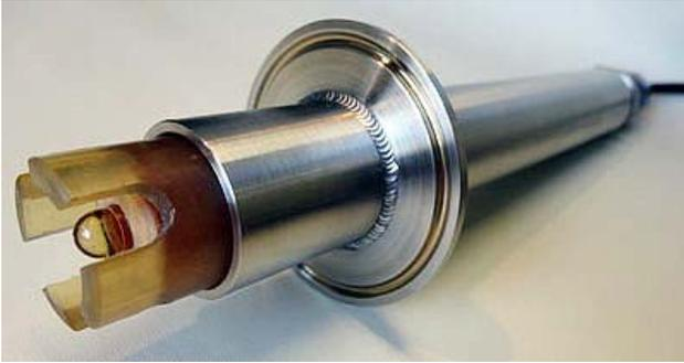
*5X31 series pH sensor installed into Tri-Clover 316SS sensor holder shown above is ready for field installation*
