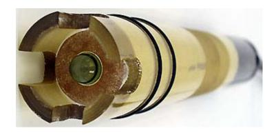
5731 Aggressive Dissolved Gas & Solvent Resistant pH sensor Close-up view of tip with 4 each "GR" thick protective times Double sealing 0-rings for integrity & safety of installation
