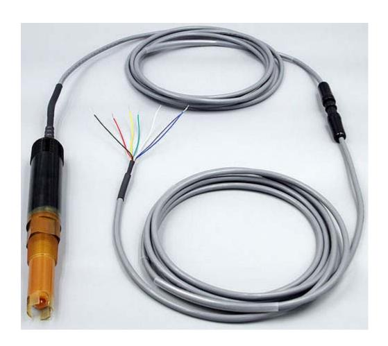
6X31 RADEL-KYNAR series pH sensor with integral preamplifier and Q7M quick disconnect snap connector interfaced with mating Q7F to tinned leads extesion cable. The Q7M/Q7F connector system is rated NEMA 6P when interfaced and suitable for rugged field use.
