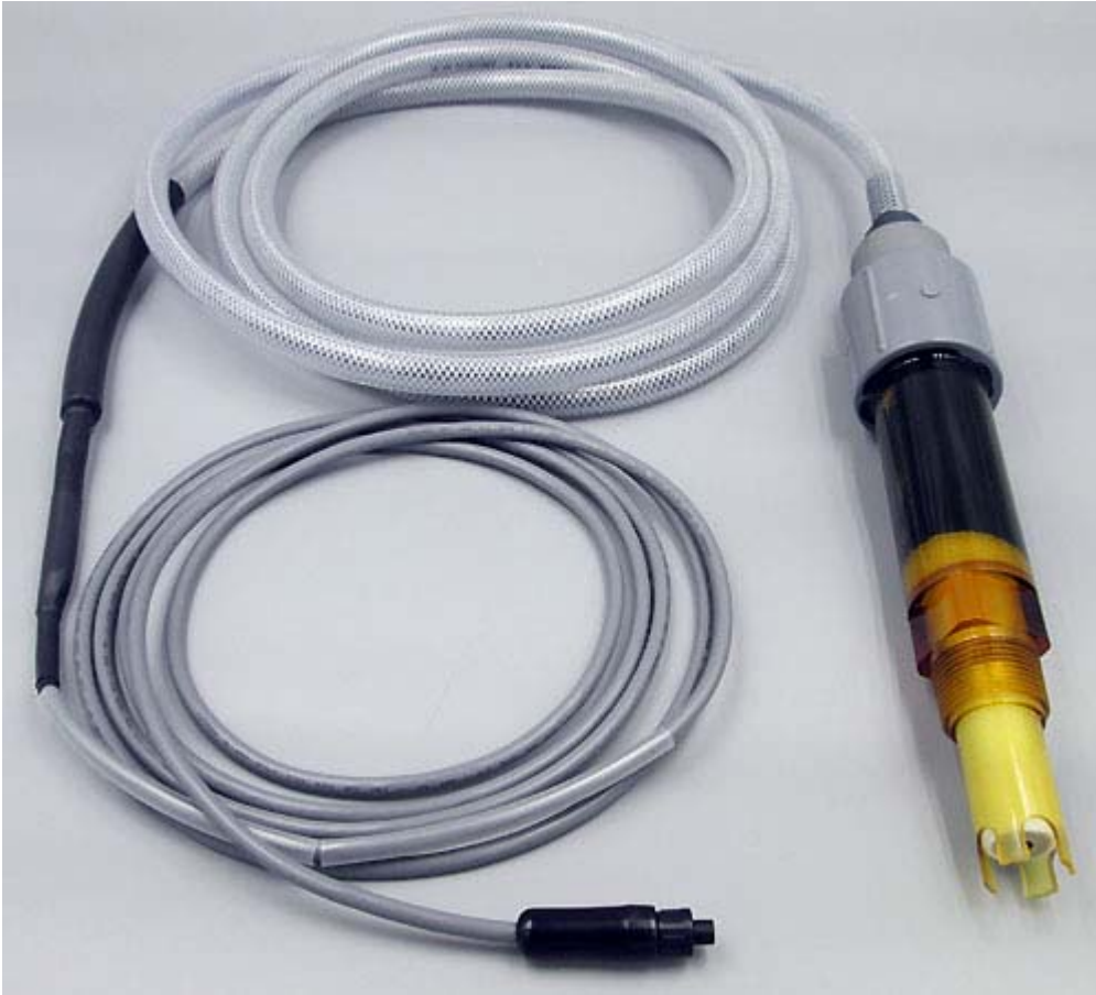
AB 6100 fluoride ion selective submersible sensor with integral preamplifier WPH waterproofing option & Q7M NEMA6P rated snap connector for use with Q7F-Xm-TL female snap to tinned lead extension cables.
