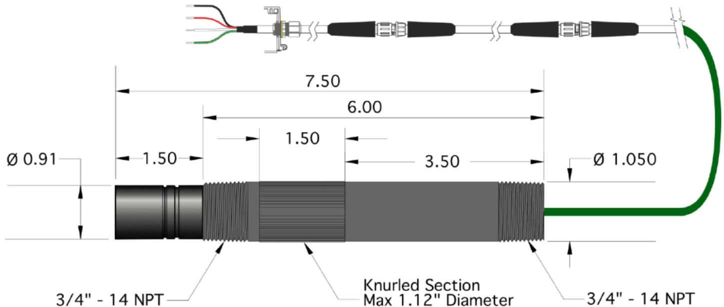
The AST-DO-UNIVERSAL smart digital MODBUS RTU dissolved oxygen sensor is a robust industrial grade sensor measures the dissolved oxygen ppm and percent (%) saturation values including salinity correction. The probe is very rugged and easy to use with automated dry in air smart calibration suitable for use in the toughest industrial, municipal, environmental and aquaculture applications.
