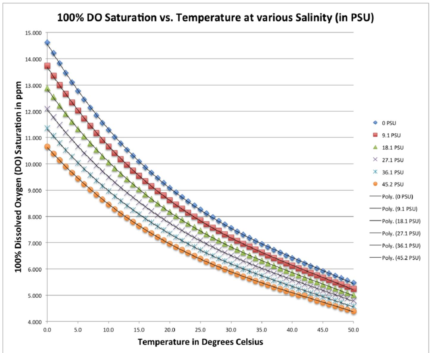
This salinity correction is only required as a correction to the computation of the %
