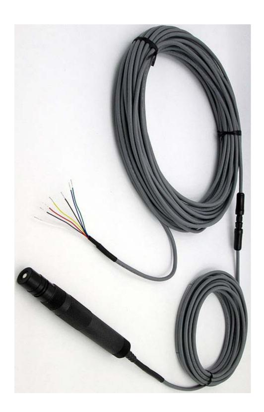
AST-DO-UNIVERSAL dissolved oxygen convertible style galvanic DO sensor in the with integral preamplifier and Q7M quick disconnect snap connector configuration. Sensor is shown interfaced to NEMA 6P rated Q7F snap to tinned leads extension cable for convenient removal from field installation for periodic cleaning, recalibration and rebuilding of the galvanic dissolved oxygen cell.
