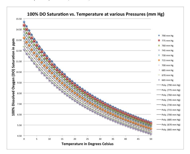
**Display Features:** Absolute mV of connected sensor, D0 ppm for 100% saturation condition at current temperature, salinity & air pressure **Salinity Correction:** From user entered PSU (PPT) salinity together with temperature and pressure to compute percent (%) saturation (see below)
