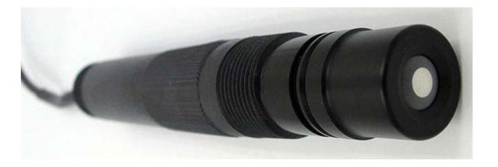
Close-Up on galvanic DO measuring cell for dissolved oxygen sensor in convertible configuration
