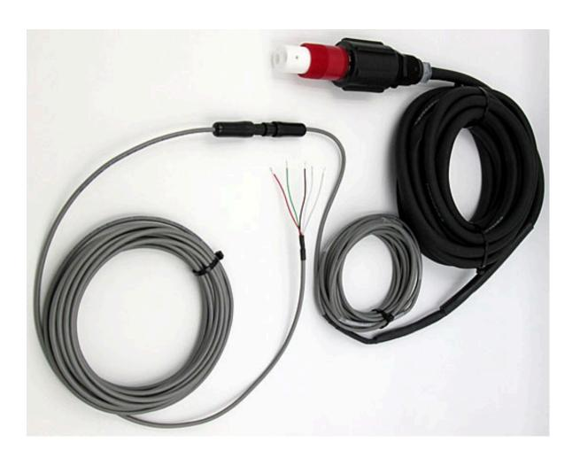
AST60 TEFLON-KYNAR Sensor in K=2.0/cm cell constant shown in a fully submersible assembly configuration complete with polypropylene (PP) waterproofing option "B" with integral NORPRENE tubing sealing for high temperature applications and Q5M/Q5F NEMA 6P rated waterproof snap connector quick-disconnect system employed
