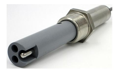
The sensor shown above has 316SS electrodes and sensor body with CPVC insulator. The 316SS electrodes are not visible as they are located inside of the two bored holes that go along the length of the insulator and are purged by the two corresponding vent holes on each side. The exposed 316SS thermowell is, however, visible which provide for fast temperature measurement to ensure accuracy conductivity values at any process condition.
