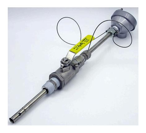
AST10 HOT-TAP Valve Retractable Assembly with  $\frac{3}{4}$ "MNPT 316SS Ball Valve in K=0.05/cm cell configuration with flared tip and safety lanyard; 316SS Electrodes with TEFLON insulator
