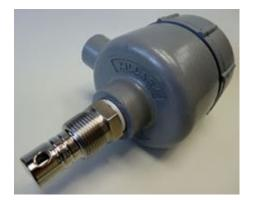
Industrial conductivity sensors for use up to 205 degrees Celsius and 500 psig suitable for measurements from 0.055 microSiemens and up to 2,000 milliSiemens. Applications supported include ultrapure water, strong acids, strong bases and concentrated electrolytes. Materials of construction include 316SS, Monel, Titanium, Hastelloy C-276 for electrodes and TEFLON, CPVC, KYNAR and PEEK for the insulator.
