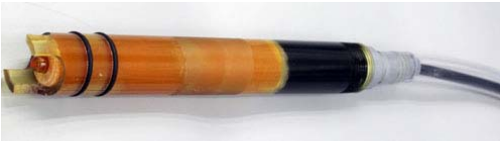
Side view of WPITC CPVC submersible option sealing assembly
