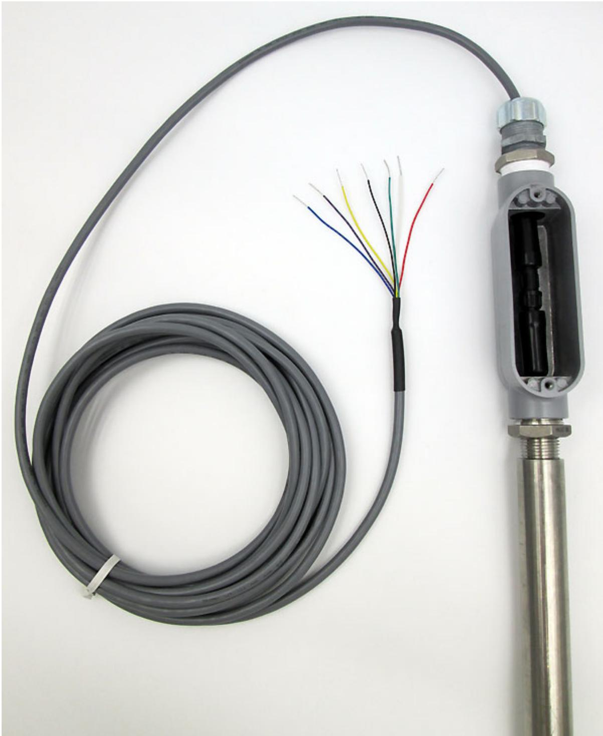
Integral bridge box installed on extension tube for easy quick disconnect sensor maintenance with Q7M/Q7F snap connector system for analog pH/ORP/ISE/DO sensors with integral preamplifiers or HiQ4M/HiQ4F snap connector system for smart digital sensors (not shown)
