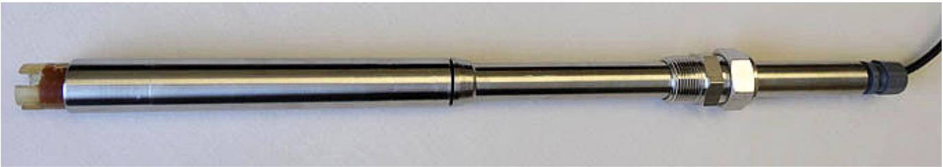
Details on just the 316SS sensor holder (on left) fitted with the short 12 inch extension tube (on right). These two parts fitted together constitute an insertion tube assembly. Also shown is the 5X31 series sensor (far left) as well as the 1" MNPT X 1.00" O.D. compression fitting and sealing cable glands. For use with the HOT-TAP valve retractable style the extension tube would be longer 36, 48 or 60 inch length as necessary for the given installation.
