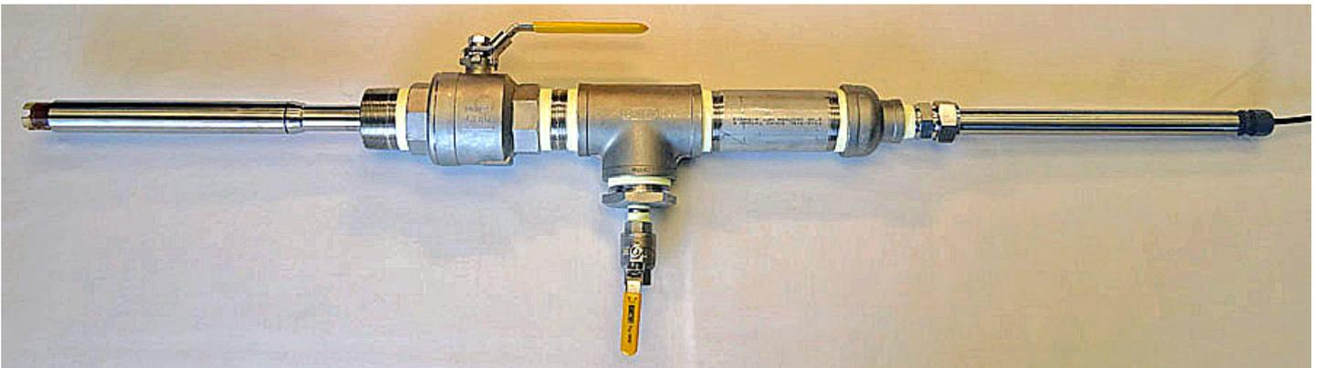
Shown above is a complete 2" NPT HOT-TAP Valve Retractable Assembly with 316SS Sensor Holder, 36 Inch Extension Tube & 5X31 Series Sensor
