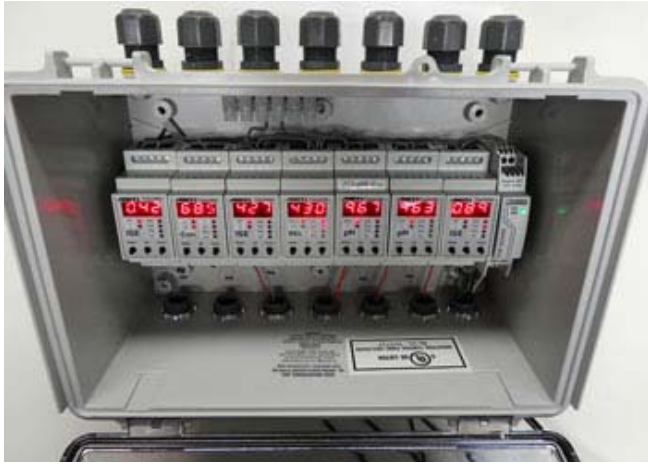
Seven Channel pH/ORP/ISE/Conductivity Assembly 3TX-7MF-ISE-CON-ISE-REL-pH-ORP-ISE-PS
