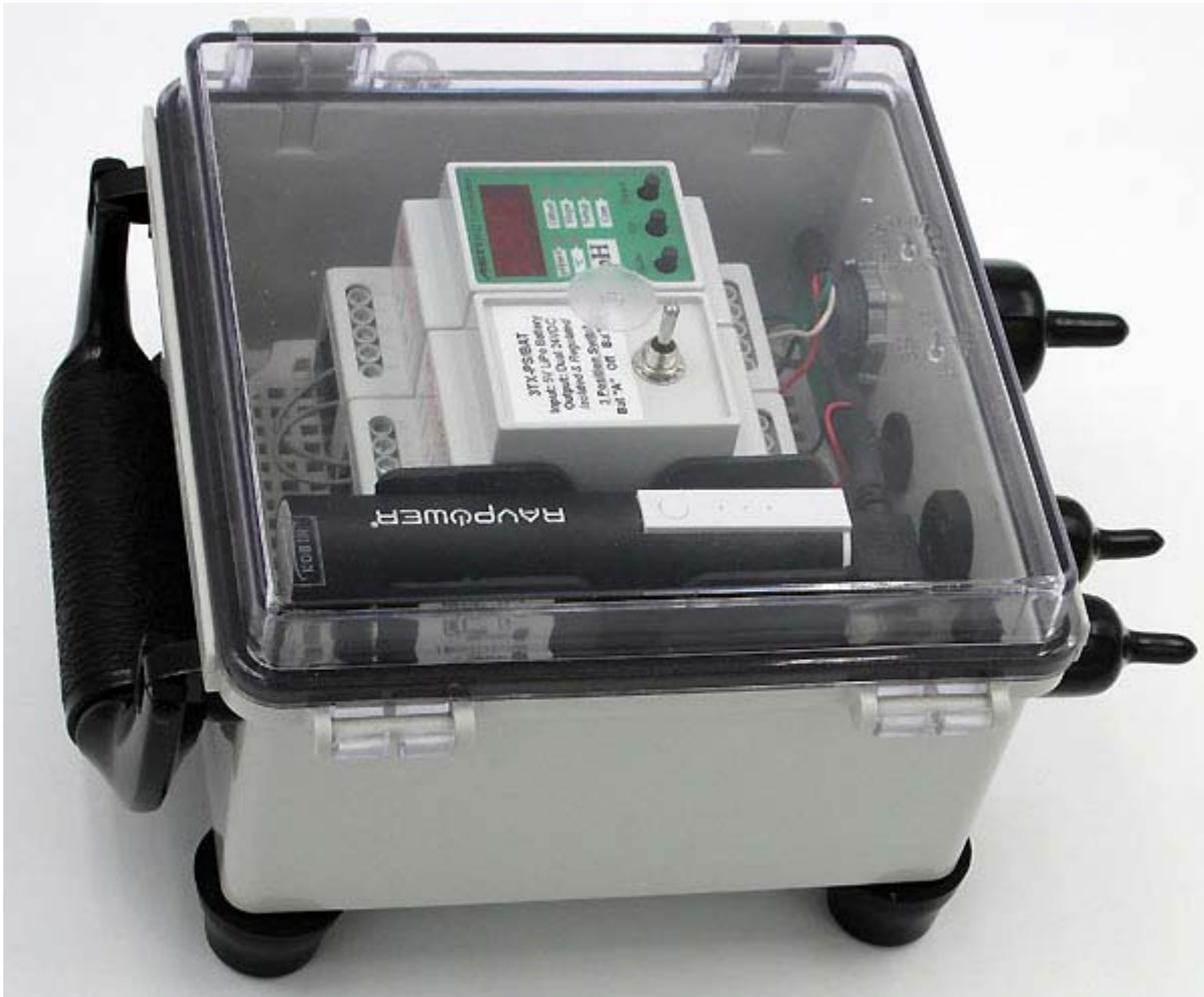
*Portable HiQ to Windows Bridge Box Close-Up detailing industrial RS-485 to USB converter.*
