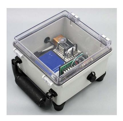
Portable HiQ to Windows Bridge Box Close-Up detailing industrial RS-485 to USB converter.
