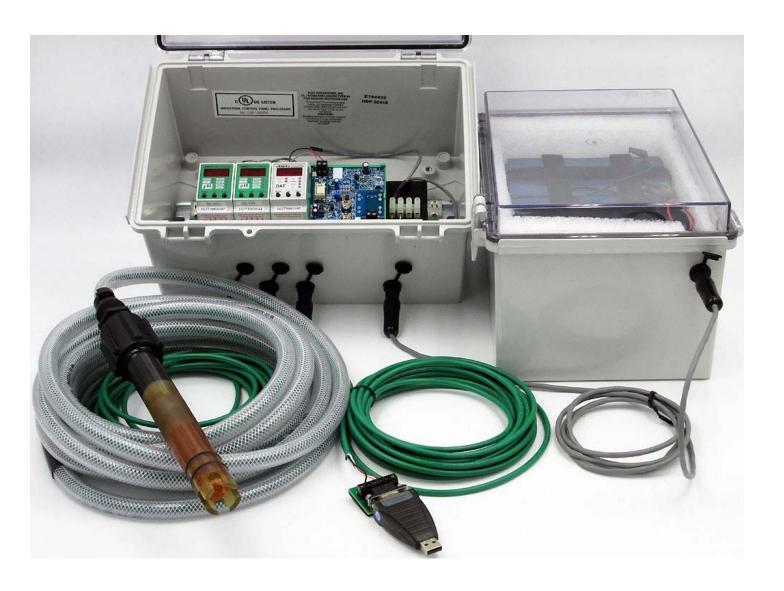
Plug & Play Submersible pH & ORP Measurement System for Intermittent Battery-Powered Operation at Remote Installations detailed as <u>Case Study # 22</u>
