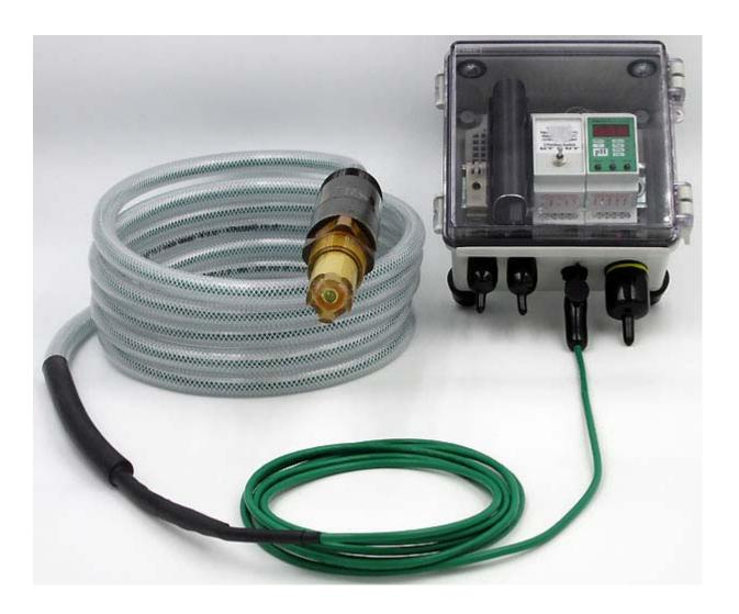
"LUNCHBOX" portable assembly with 6700mAH rated LiPo battery & Smart Digital ZEUS™ pH sensor interfaced via HiQ4FP female panel connector to mate with HiQ4M male sensor snap connector
