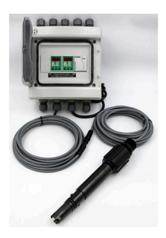
Complete assembly showing smart digital dual pH/ORP all-in-one sensor with HiQ7M snap connector interfaced to HiQ7F female snap to tinned lead extension cable which is terminated to two (2) each 3TX-HiQ-pH transmitters. One of the modules displays and outputs the pH while the other module displays and outputs ORP from the connected smart digital dual pH/ORP all-in-one sensor.
