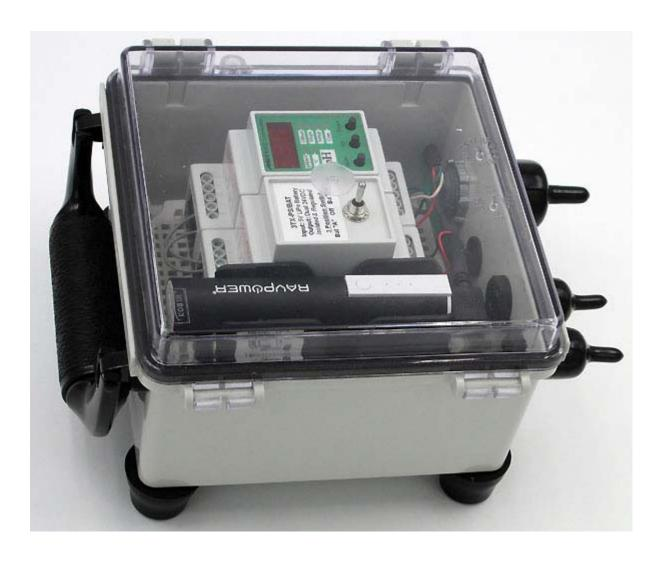
Portable HiQ to Windows Bridge Box Close-Up detailing industrial RS-485 to USB converter.
